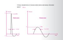
p, and p, are the maximum positive and negative pressure. The amplitude p+ of shock and pressure waves differs by a factor of 10-100.
